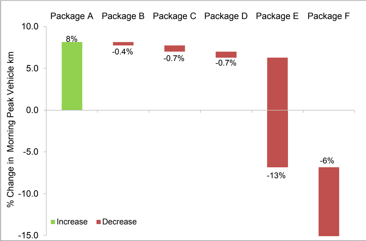
Figure 7.3 Change in London morning peak hour vehicle kilometres, 2015 to 2041 for packages A to F.
